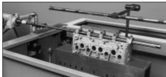
Cylinder head being honed on CH-100 Honing Machine with a hand fed Porta-Hone.
